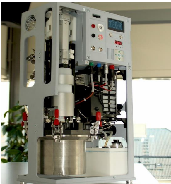
Figure 2. Hydropaste and 100 W PEM fuel cell by Fraunhofer IFAM
