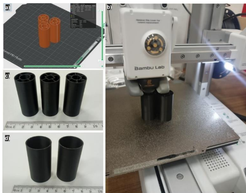
Figure 4. Fabrication process using 3D Printing: (a) Bambu lab software; (b) Printing process; (c) Multi-cell tube; (d) shell tube
