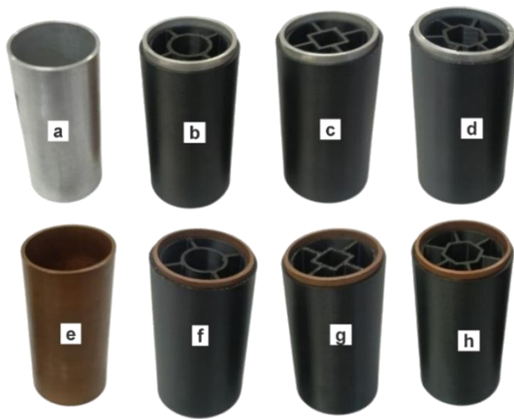
Figure 5. Crashworthiness specimens: (a) Al-T; (b) CB-Al-C; (c) CB-Al-S; (d) CB-Al-H; (e) Cu-T; (f) CB-Cu-C; (g) CB-Cu-S; (h) CB-Cu-H
