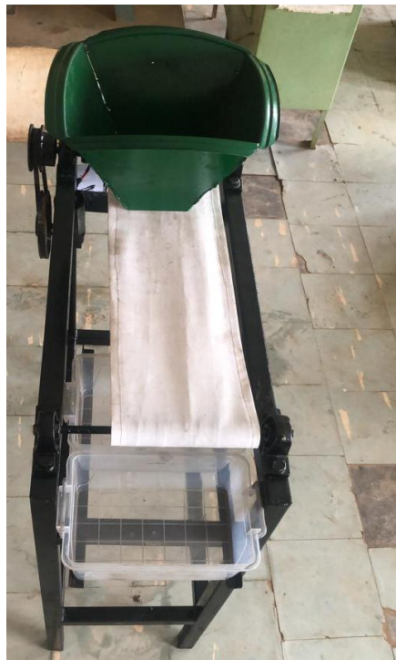
Figure 3. Picture of the developed permanent induced magnetic separator.
