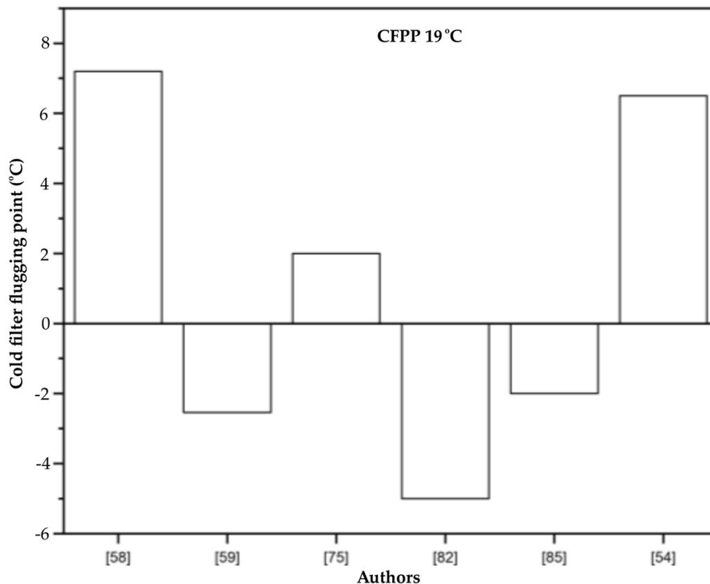
Figure 10. Cold filter plugging point of Biodiesel WCO
