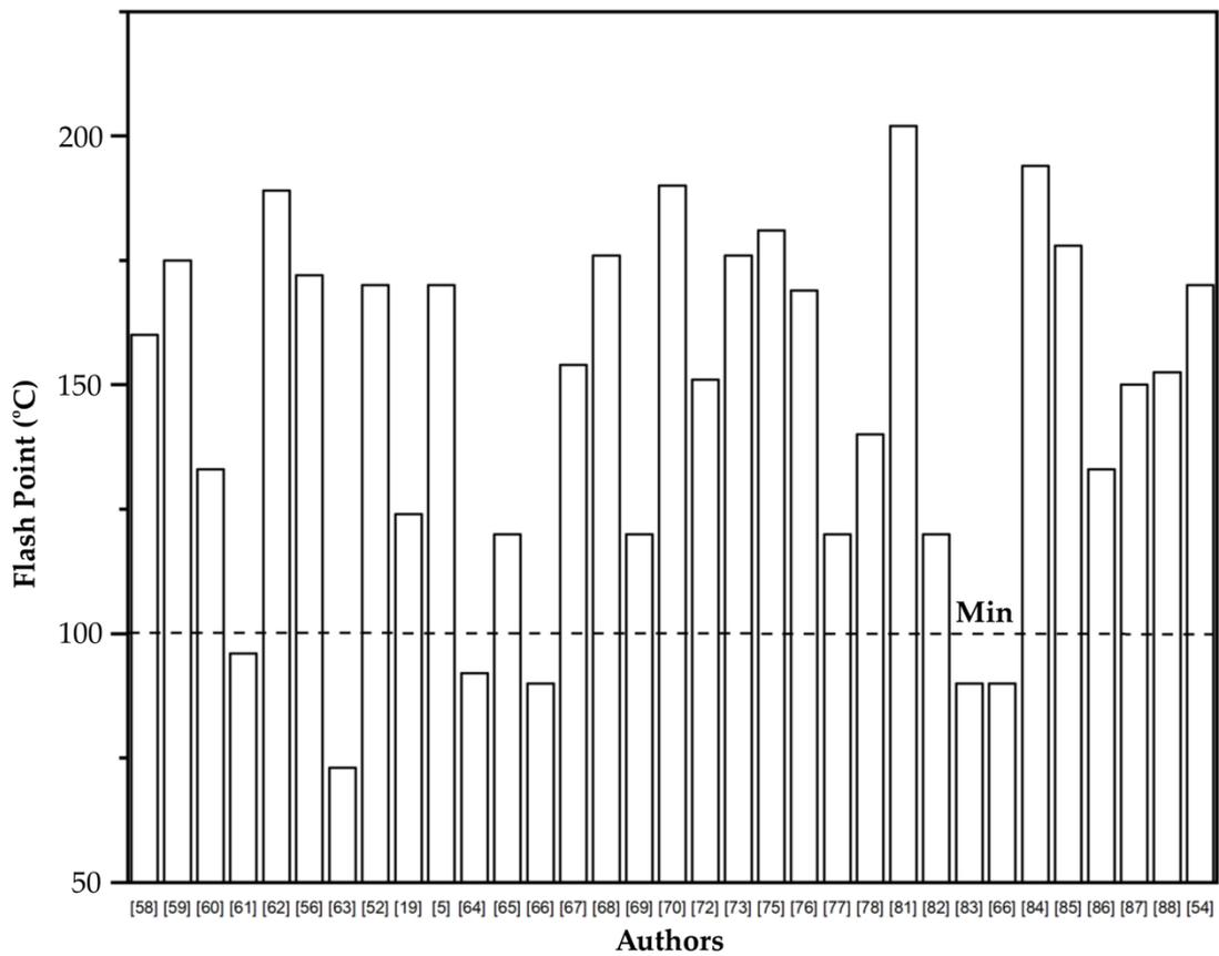
Figure 5. The flash point of WCO biodiesel
