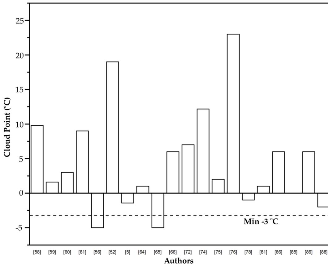
Figure 9. Cloud point of biodiesel WCO
