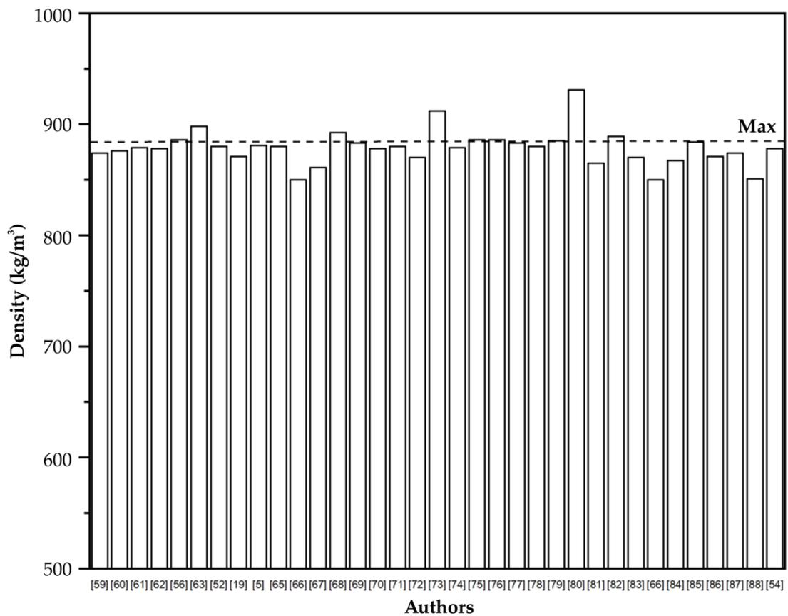
Figure 3. Density of biodiesel WCO
