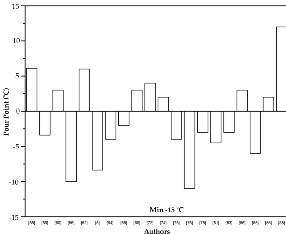
**Figure 6.** Pour point of WCO biodiesel
