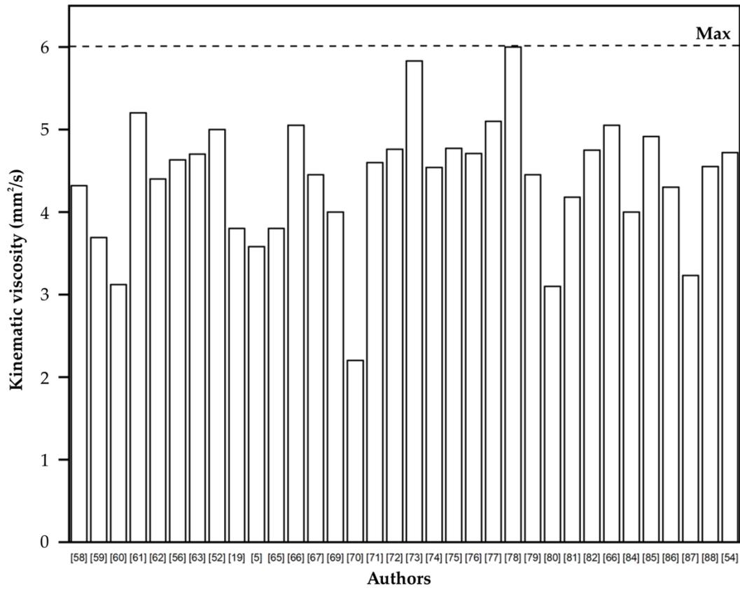
Figure 2. Kinematic viscosity of produced biodiesel WCO
