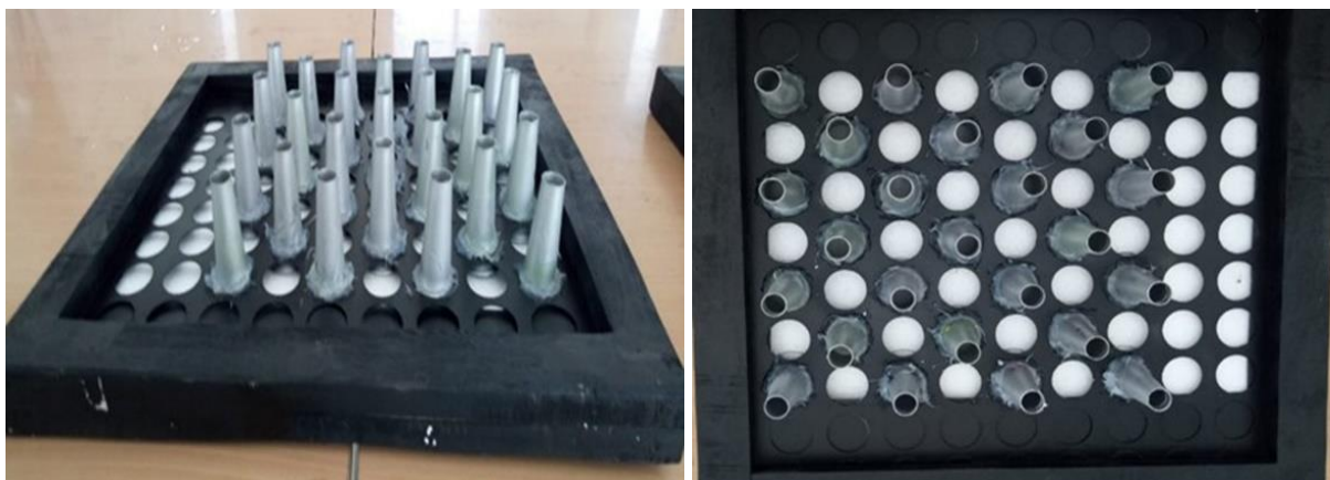
Figure 6. Nozzle arrangement plate with a diameter of 30 mm
