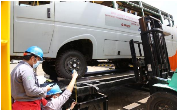
Figure 19. Forklift speed measurement for lifting platform
