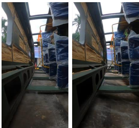
Figure 22. Visual residual space against the vehicle wall right when the vehicle hits the floor seen from the front
