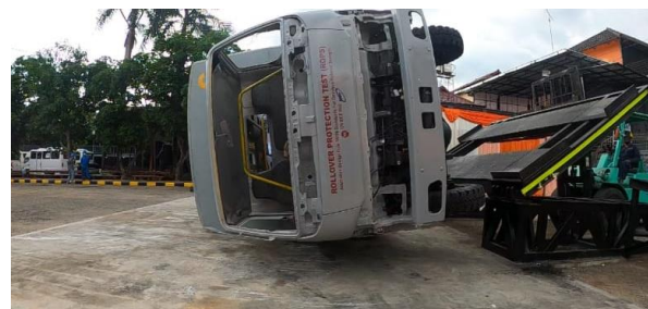
Figure 24. Visual residual space against the vehicle wall right when the vehicle hits the floor seen from the outside of the front vehicle
