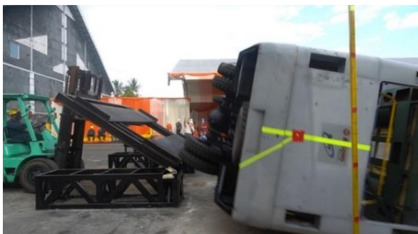
Figure 21. The lowest position of the Centre of Gravity man-hauler after it toppled
