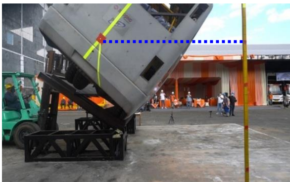
Figure 20. Man-hauler lifts before toppling with the Centre of Gravity at its highest point
