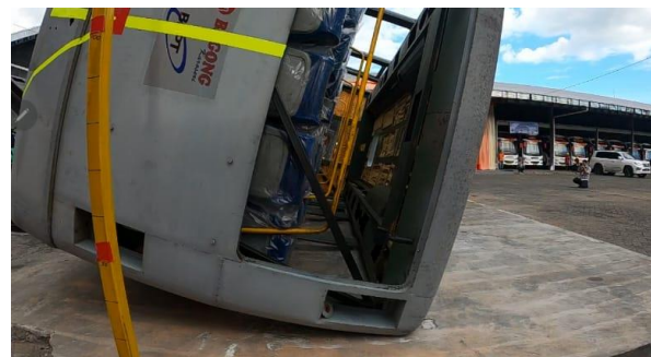
Figure 25. Visual residual space against the vehicle wall right when the vehicle hits the floor seen from outside the rear of the vehicle
