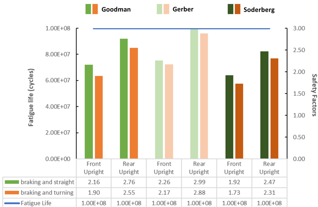
Figure 5. Fatigue simulation results for designing the front and rear upright
