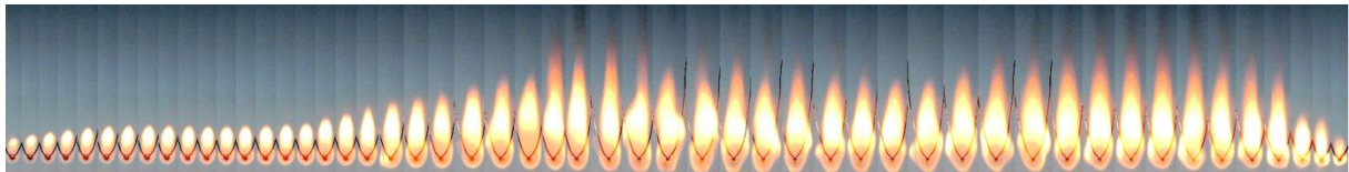
Figure 3. Droplet diffusion flame of crude castor oil without catalyst
