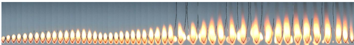
Figure 4. Droplet diffusion flame of crude castor oil with catalyst
