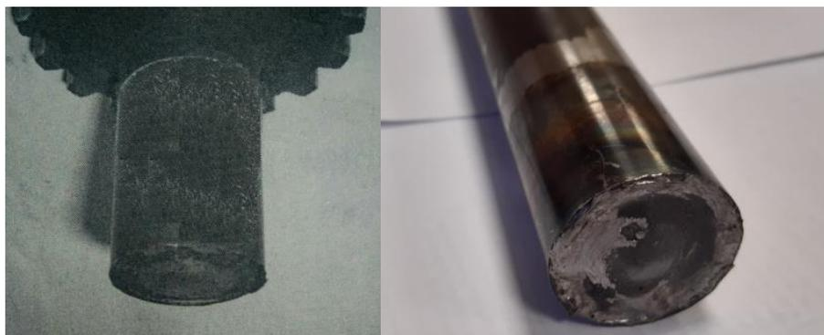
**Figure 2.** Low-cycle failure of elastic transmission bars when operating in off-design modes (in resonant modes causing plastic deformations)
