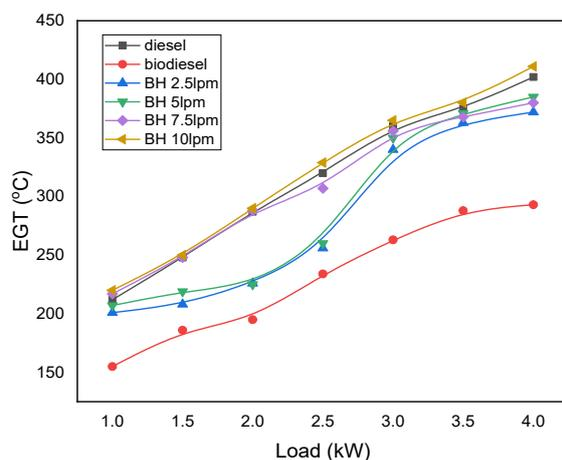
Figure 3. Variation of EGT against engine load
