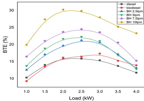
**Figure 5.** Variation of engine BTE on engine load
