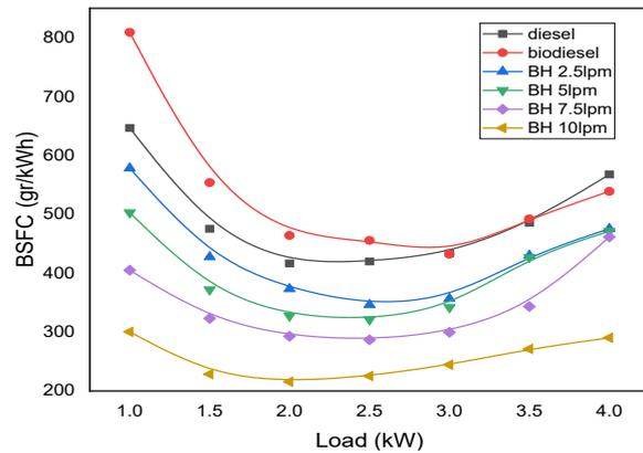
**Figure 6.** Specific fuel consumption on engine load
