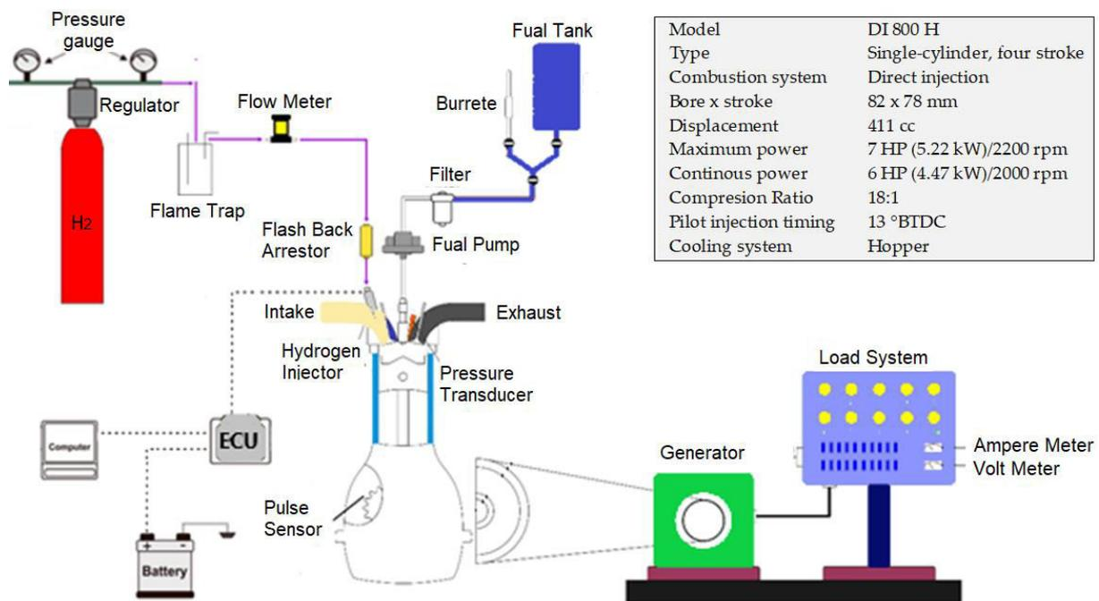
Figure 1. Schematic of testing equipment
