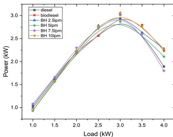
Figure 4. Power against engine load
