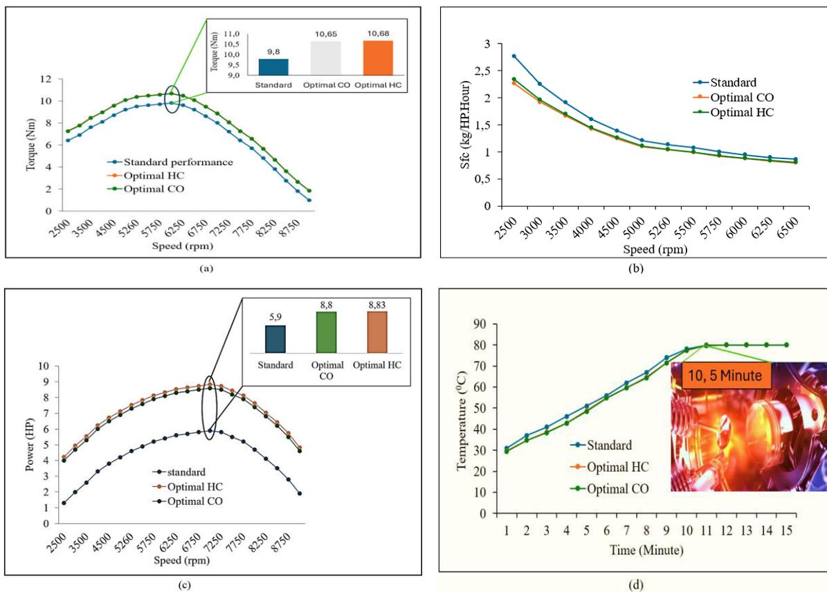
**Figure 5.** Performance characteristics, a) torque vs speed, b) Specific fuel consumption (Sfc) vs speed, c) power vs speed, d) time to temperature increase
