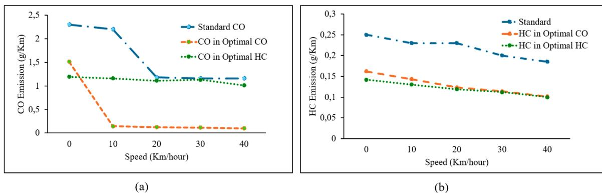
Figure 6. Emission characteristics, a) CO characteristics vs speed in optimal CO, b) HC characteristics vs speed in Optimal HC
