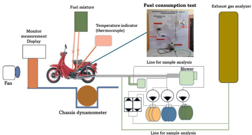
**Figure 2.** Experimental set up with fuel consumption test
