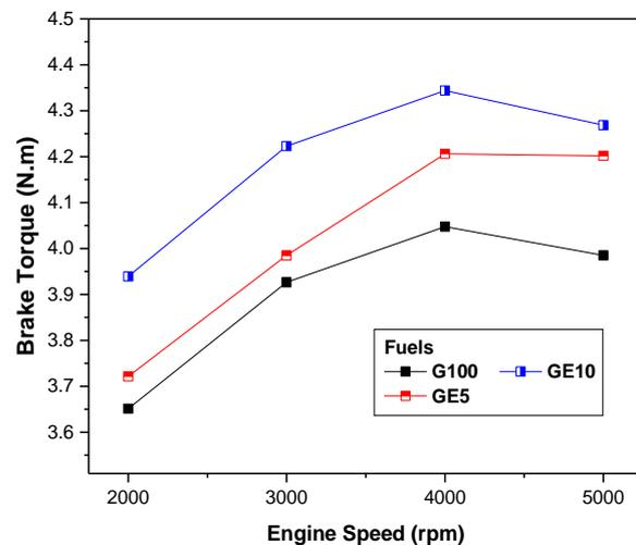
Figure 5. Brake torque of gasoline engine fueled by gasoline-mangrove biofuel
