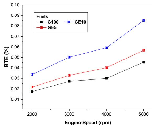
**Figure 8.** BTE of gasoline engine fueled by gasoline-mangrove biofuel
