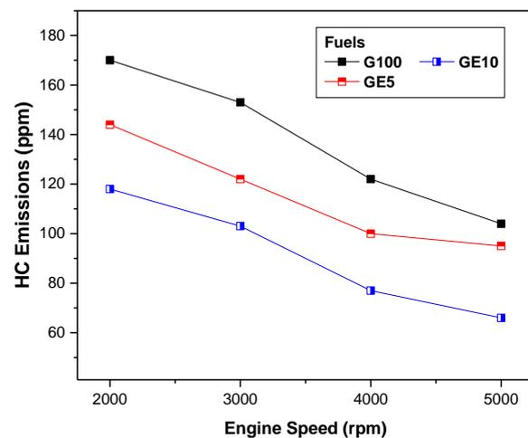
Figure 11. HC emissions from the use of gasoline engines fueled by G100, GE5, and G10
