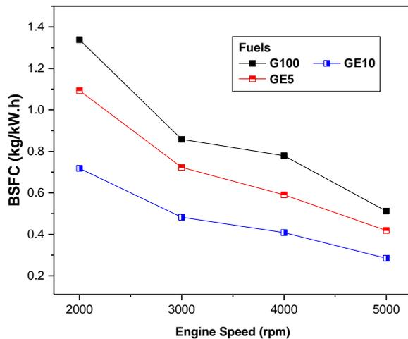
**Figure 7.** Brake-specific fuel consumption (BSFC) of gasoline engine using gasoline-mangrove biofuel
