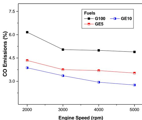
Figure 10. CO emissions of gasoline engines fueled by G100, GE5, and GE10
