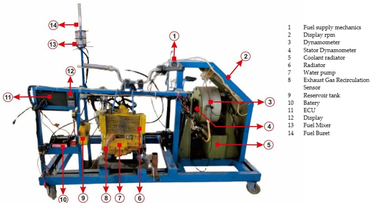
**Figure 3.** 150 cc gasoline engine with water cooling system
