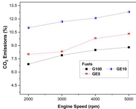
**Figure 12.** CO<sub>2</sub> emissions measured using G100, GE5, and GE10 fuels
