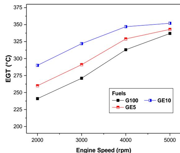
**Figure 9.** EGT of gasoline engine fueled by gasoline-biofuel mangrove
