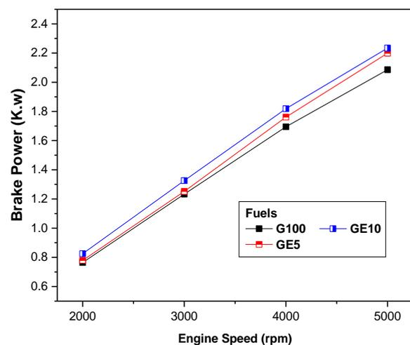
Figure 6. Brake power of gasoline engine fueled by mangrove gasoline-biofuel
