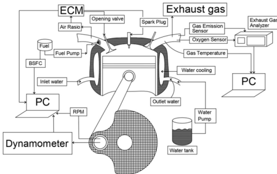
**Figure 4.** Integration of gasoline engine-dynamometer-gas analyzer setup
