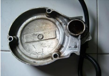
Figure 9. Release cylinder holder
