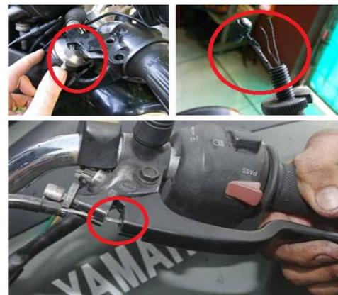
Figure 1. Damage on mechanical clutch
