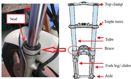
**Figure 1.** Schematic view of telescopic front fork (TFF) of motorcycle [1]
