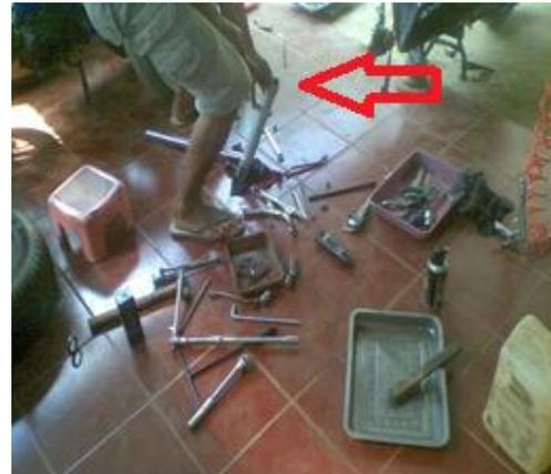
**Figure 2.** Hazardous front fork seal removal
