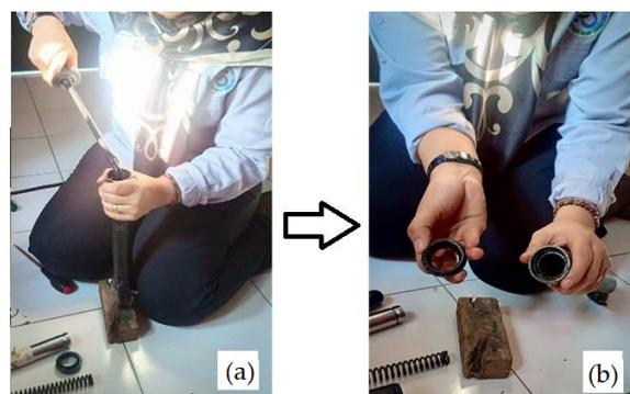
Figure 5. Photographic view of product testing by the author: the process of removing seal (a) and removed seal (b)
