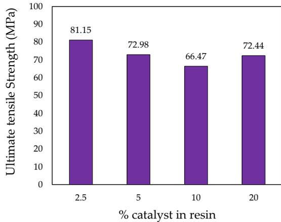
Figure 7. Ultimate tensile strength to % catalyst in resin
