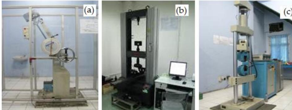
**Figure 4.** Test equipment: (a) impact test equipment, (b) bending test equipment, and (c) tensile test equipment
