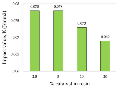
**Figure 5.** Impact to % catalyst in resin, complete data is given in **Appendix 1 (Table 1)**
