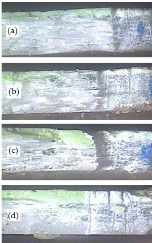
Figure 8. Photograph view of specimens fracture with catalyst composition: (a) 2.5% (b) 5% (c) 10% and (d) 20%.
