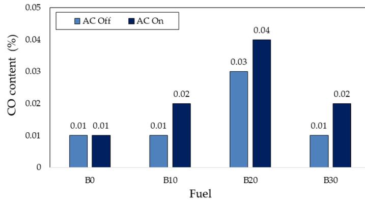
Figure 5. Comparison of CO emission with and without AC load.
