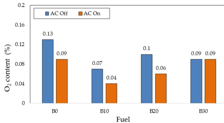
Figure 7. Comparison of O<sub>2</sub> content with and without AC load.
