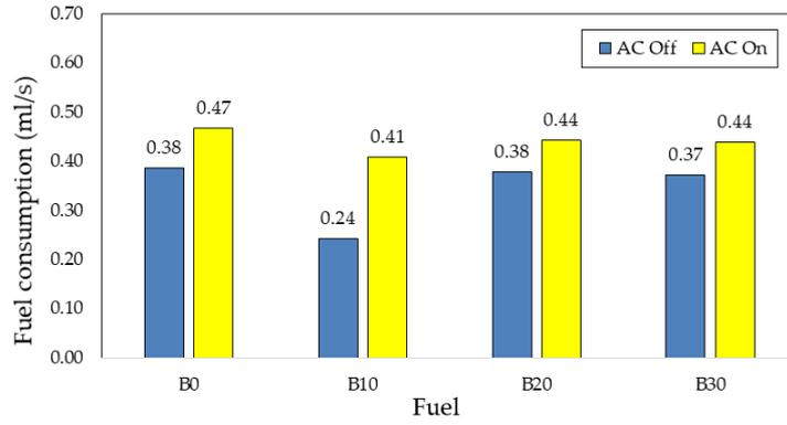
Figure 4. Comparison of fuel consumption with and without AC load.
