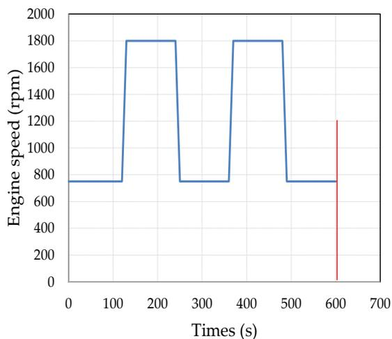
**Figure 3.** The evolution of engine speed during the test (The vertical red line in the 600th second indicates the cease of fuel pump operation)
