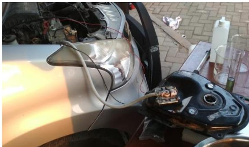
**Figure 1.** Special fuel tank for cassava biogasoline experimental test
