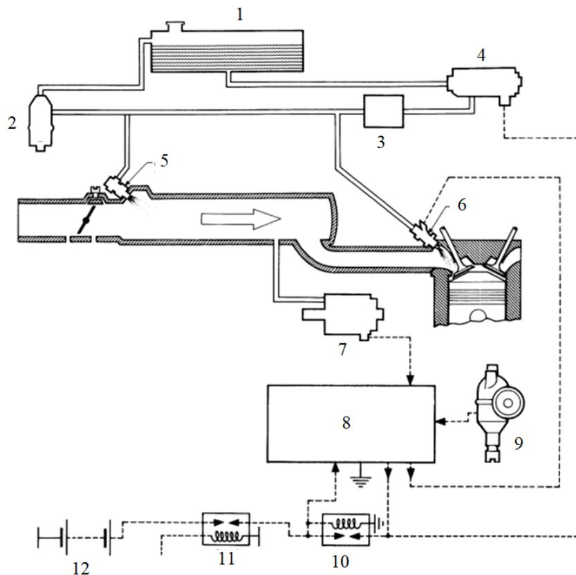
**Figure 2.** EFI fuel system: (1) fuel tank, (2) regulator, (3) filter, (4) fuel pump, (5) cold start injector, (6) injector, (7) pressure sensor, (8) ECU, (9) distributor, (10) fuel pump relay, (11) main relay, dan (12) battery.
