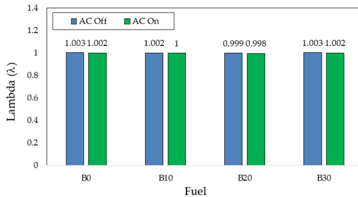
Figure 6. Comparison of lambda value with and without AC load.
