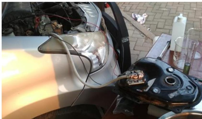
**Figure 1.** Special fuel tank for cassava biogasoline experimental test
