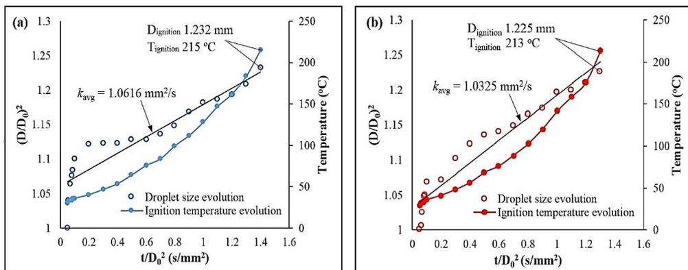
**Figure 2.** The evolution of droplet: (a) without catalyst and (b) with catalyst
