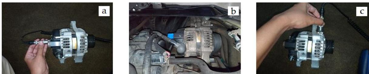
Figure 2. Frequency response function measurement
