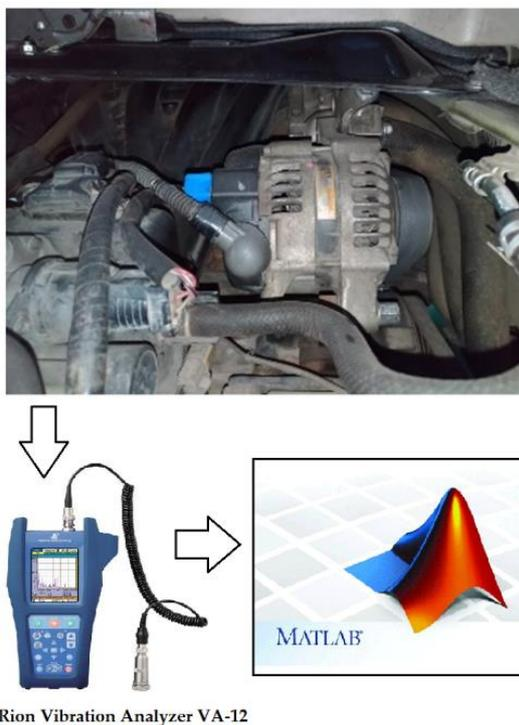
**Figure 3.** Set-up experiment
