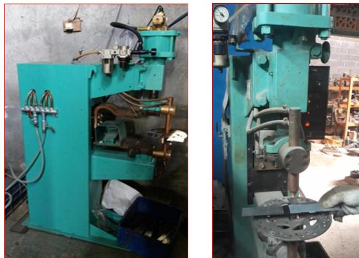
**Figure 4.** RSW machine 35 kW capacity
