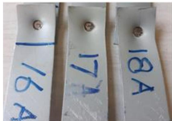
Figure 8. Pull-out failure mode for iteration 16, 17 and 18
