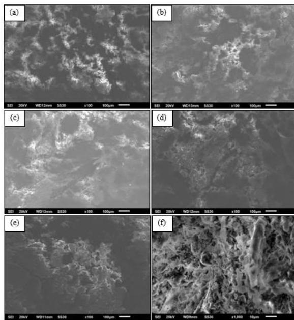
**Figure 8.** Scanning electron microscopy (SEM) images of (a-e) specimen A-E, (f) genuine part
