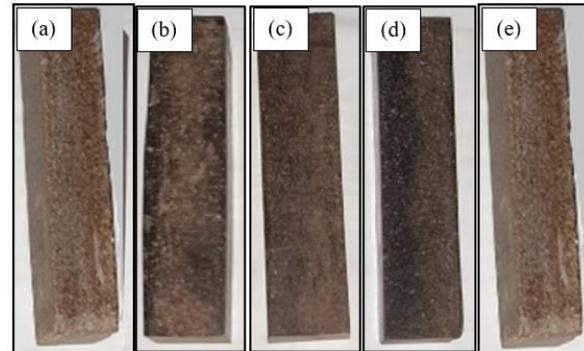
Figure 6. Specimens A-E for testing: hardness, coefficient of friction, wear and microstructure
