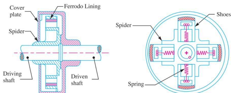
Figure 1. Centrifugal clutch [18]
