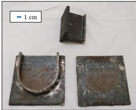
Figure 3. Mold for made specimen
