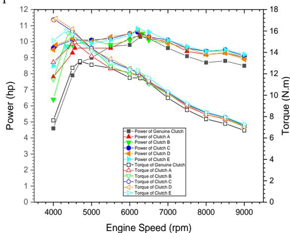
Figure 10. Power and torque at each engine speed from chassis dyno test results
