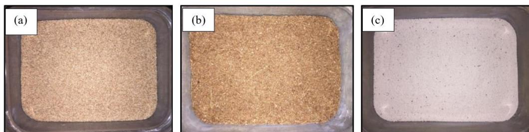
**Figure 2.** Powder materials for composite mixtures: (a) wood, (b) coconut fiber, (c) shellfish shell
