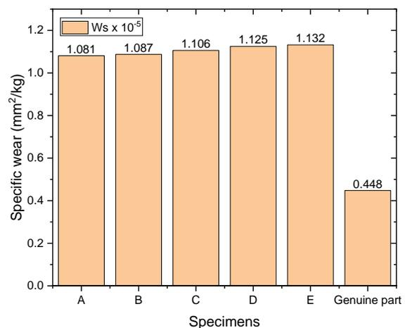
**Figure 9.** Specific wear of specimens.
