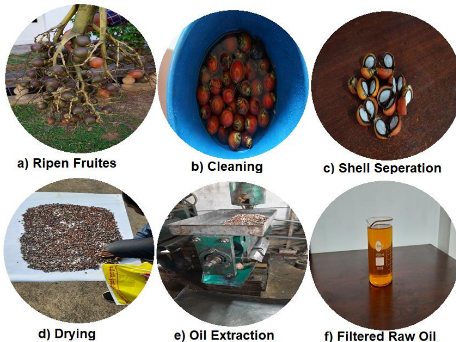
Figure 2. (a-f) Oil extraction process from wodyetia bifurcate
