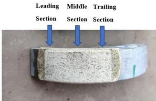
**Figure 6.** Test-sections of the clutch liner
