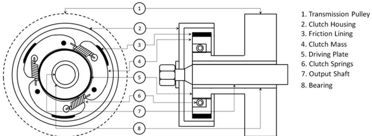
Figure 1. Centrifugal clutch
