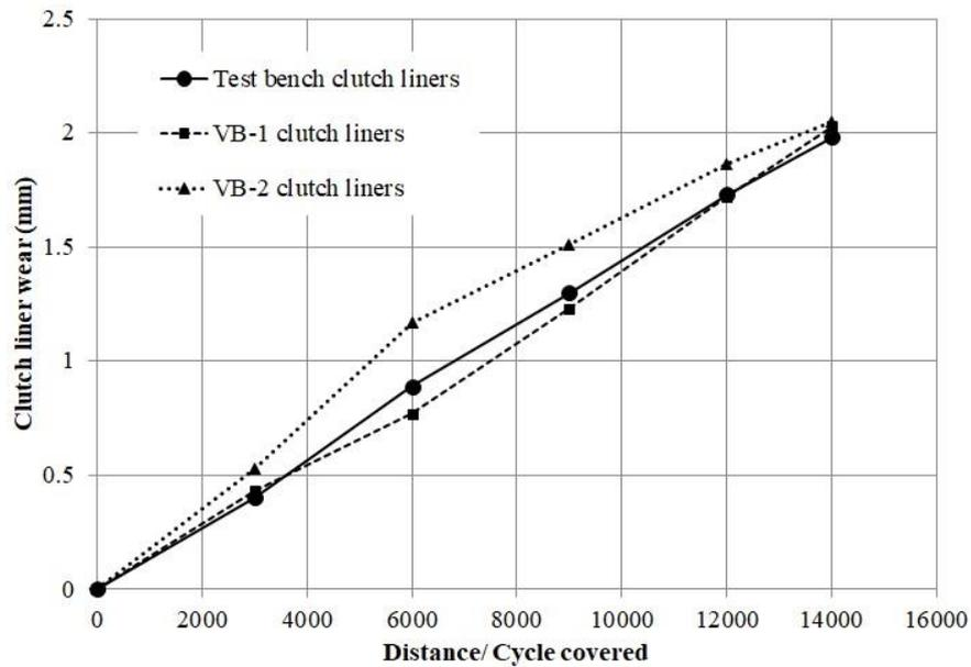
Figure 9. Wear of vehicle clutch liners and test bench clutch liners
