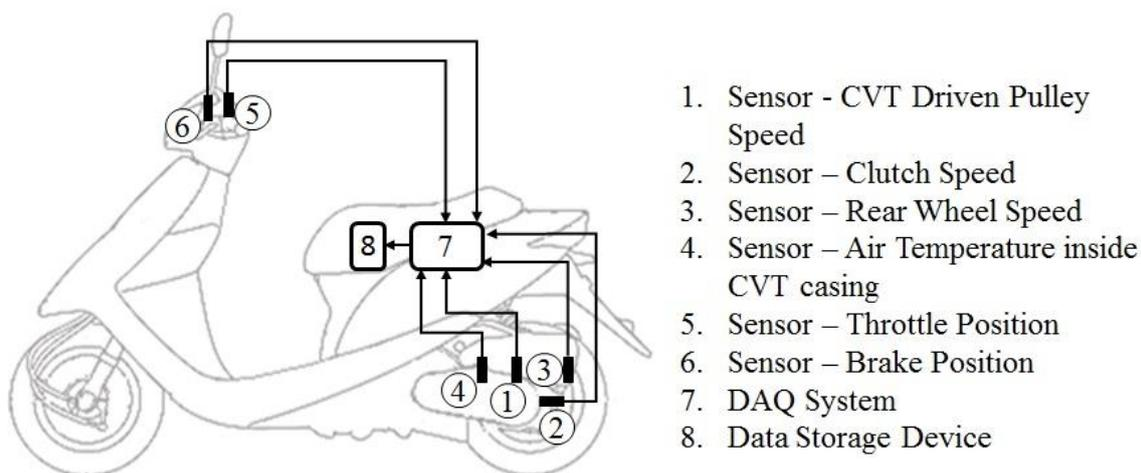
**Figure 2.** Representation of pilot vehicle with instrumentation layout
