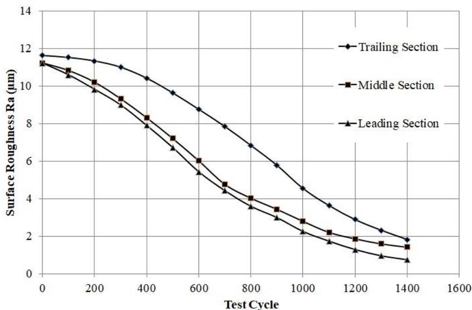
**Figure 7.** Variation in average surface roughness for three test sections of clutch liner
