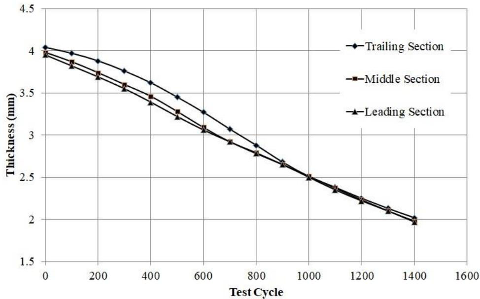
Figure 8. Variation in thickness for three test sections of clutch liner
