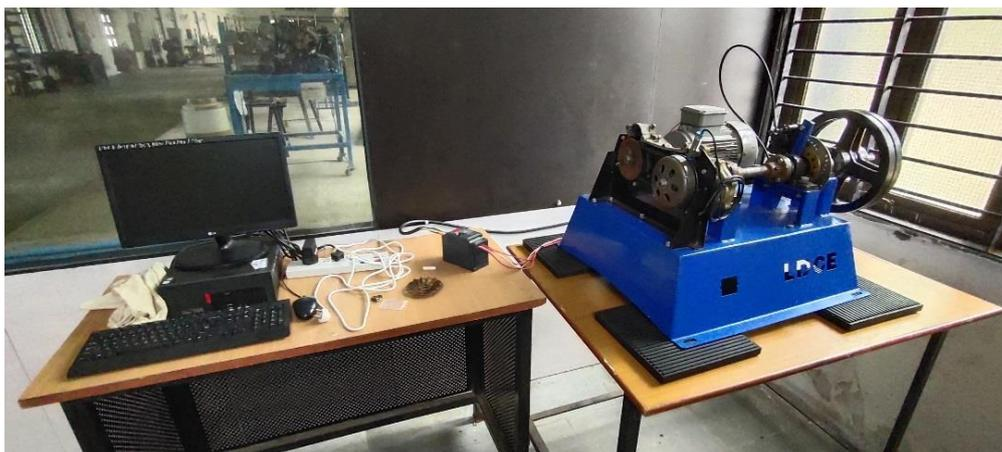
**Figure 5.** Experiment Setup for centrifugal clutch test
