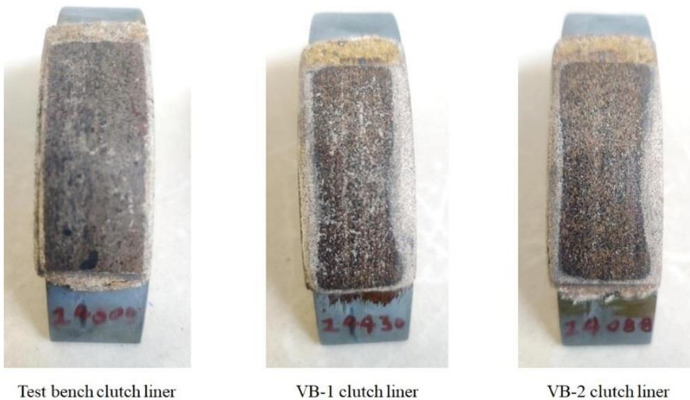
Figure 10. Clutch liners after 1400 test cycles on test bench and equivalent distance on vehicle
