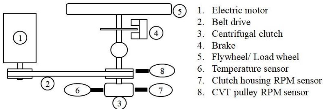
**Figure 4.** Schematic of centrifugal clutch test bench
