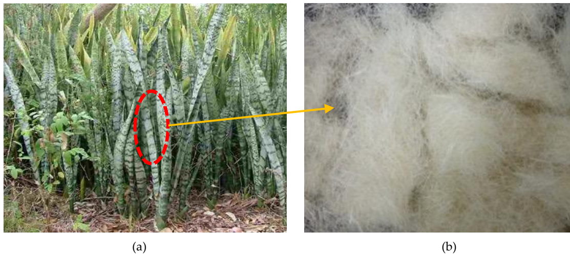
Figure 1. Natural resource fibre reinforced Vinyl Ester as STF/VE bio-composites: (a) Sansevieria Trifasciata, (b) Sansevieria Trifasciata fibre (STF)
