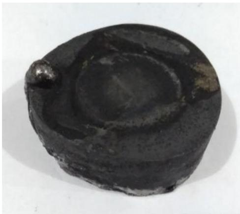
**Figure 4.** Induction hardening failure in specimen 4
