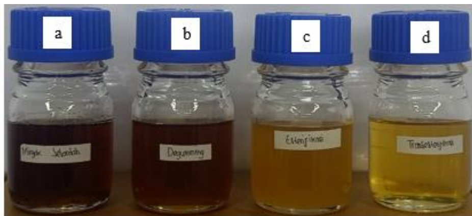
Figure 6. (a) Waste cooking oil; (b) Degumming product; (c) Esterification product; (d) Transesterification product
