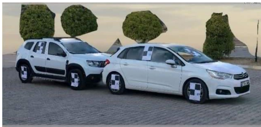
Figure 5. Textured model obtained by using close-range photogrammetry method
