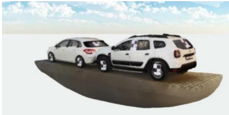
Figure 6. Point cloud obtained by using laser scanner method [5]
