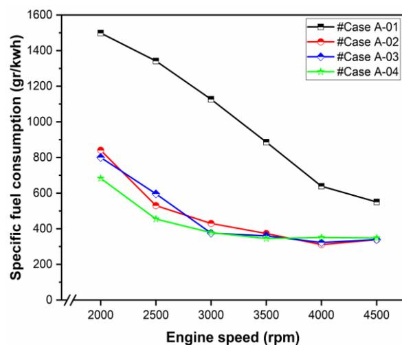
Figure 8. Specific fuel consumption vs. engine speed
