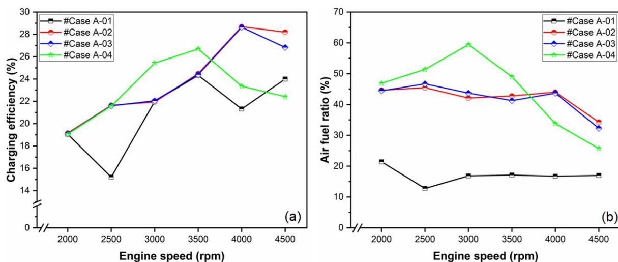
Figure 9. (a) Charging efficiency and (b) air-fuel ratio (A/F) vs. engine speed for pressure variations
