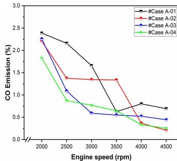
Figure 6. CO Emissions vs. engine speed
