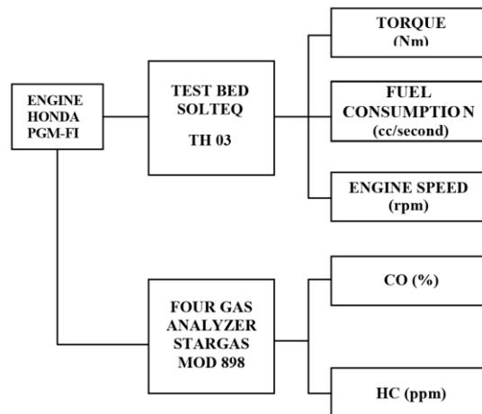
Figure 3. Schematic of combustion and emissions test performance with ethanol addition
