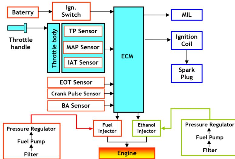
Figure 2. Schematic of modification of the fuel system with the addition of ethanol
