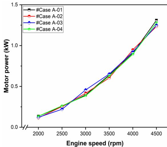
Figure 5. Power vs. engine speed for pressure variations
