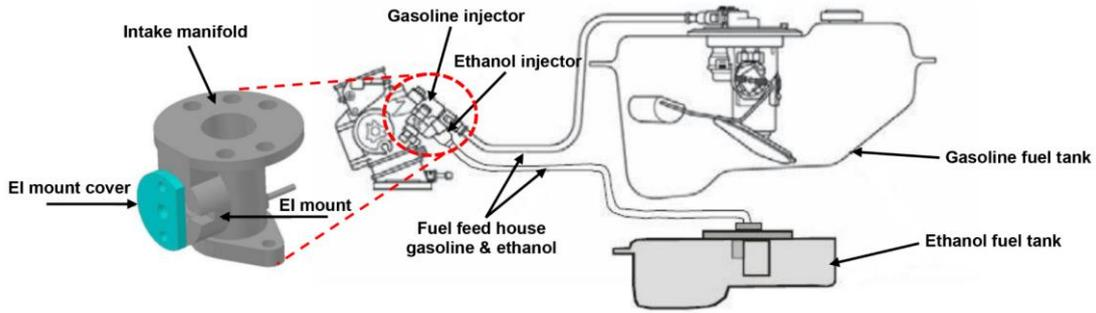
Figure 1. EFI system and intake manifold modification with the addition of ethanol injector
