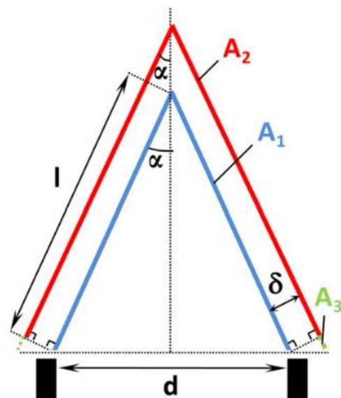
Figure 3. Illustration of cone bunsen flame angle [36], [37]
