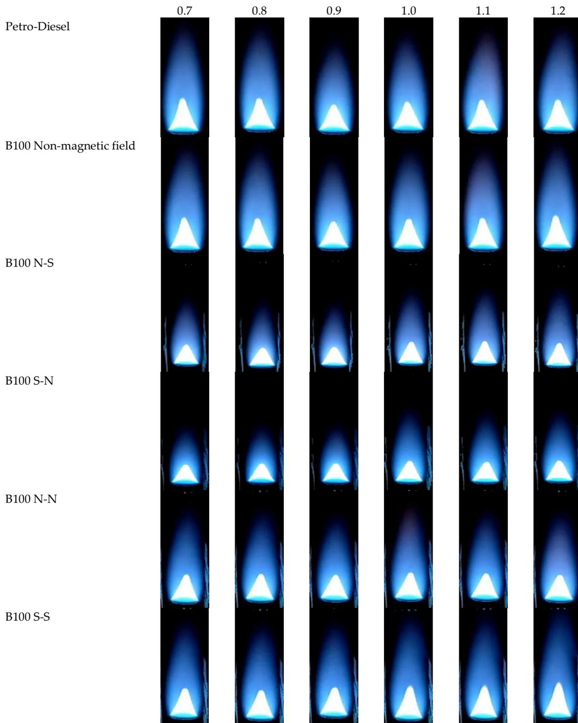
**Figure 4.** Flame with magnetic fields variation and equivalent ratio
