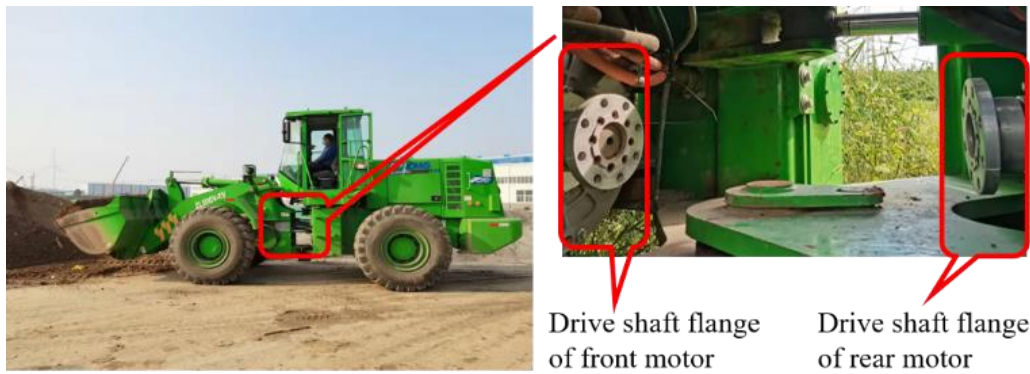
Figure 7. An electric wheel loader with two motors
