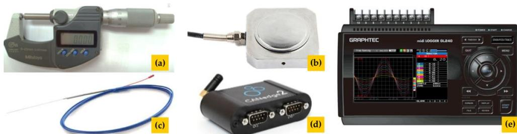
Figure 1. Measuring instruments: (a) Micrometer (0-25mm range); (b) Brake pedal force sensor; (c) K-type thermocouple; (d) CANedge2 logger; (e) Graphtec data logger
