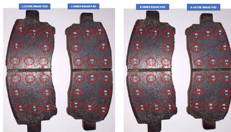
Figure 3. Brake pad measurement point selection
