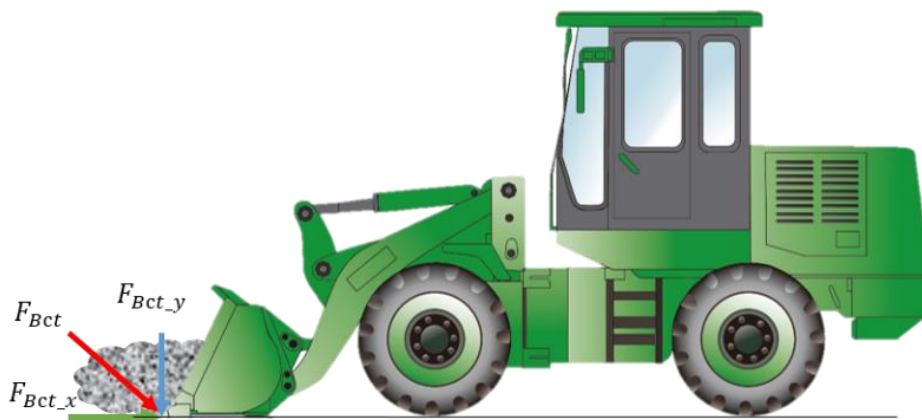
Figure 2. A force generated when the bucket touches against ground in shoveling condition
