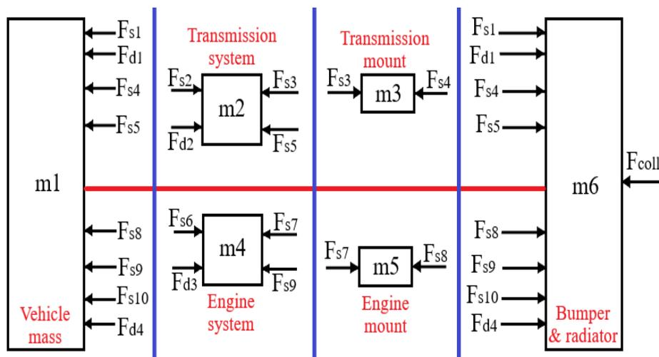
Figure 4. Schematic diagram of the modified Kamal model
