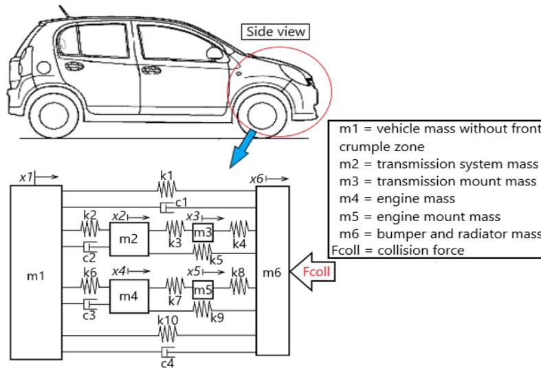
Figure 3. Free-body diagram of the crumple zone modeling
