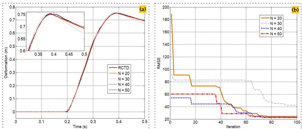
**Figure 5.** The outcome of varying the number of agents,  $N$ : (a) Deformation; and (b) Root means square error
