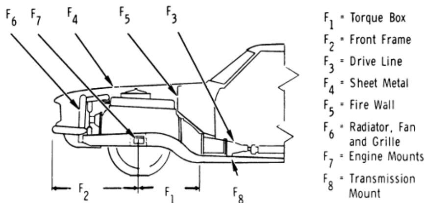
Figure 2. The dynamic forces acting on the front crumple zone [13]
