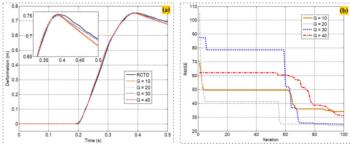
**Figure 7.** The outcome of varying the gravitational constant,  $G$ : (a) Deformation; and (b) Root means square error
