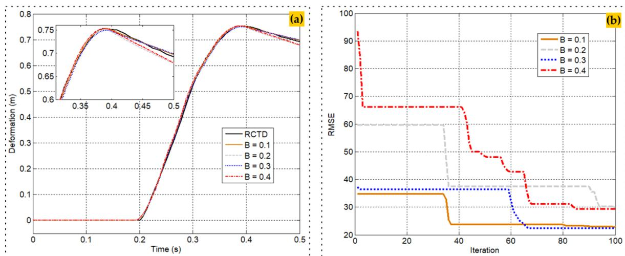
**Figure 6.** The outcome of varying the beta parameter,  $\beta$ : (a) Deformation; and (b) Root means square error
