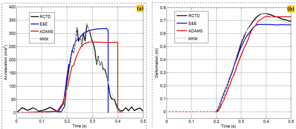
**Figure 10.** Comparison with others model: (a) Acceleration; and (b) Deformation
