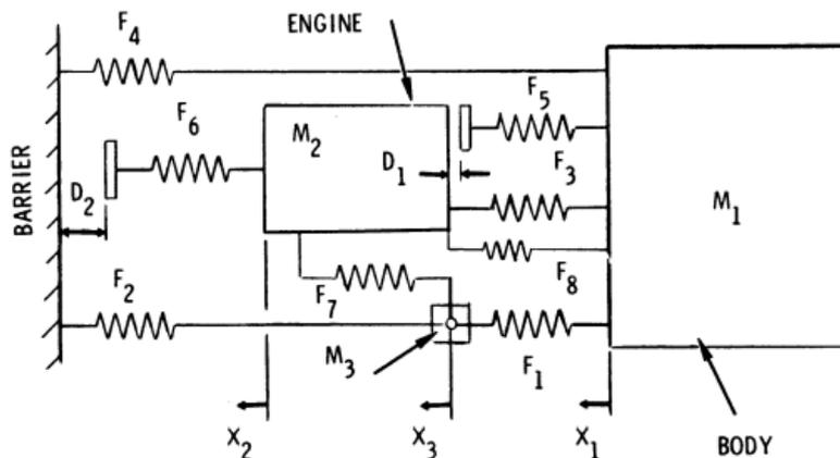
Figure 1. Mathematical model of a barrier impact [13]
