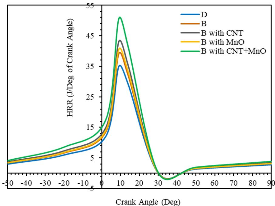
Figure 6. Relationship between heat release rate (J/DCA) with crank angle variations (degree)
