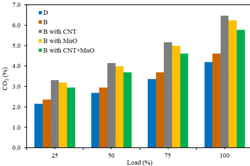
Figure 11. Exhaust emission of Carbon dioxide (%) variation for the different load (%)
