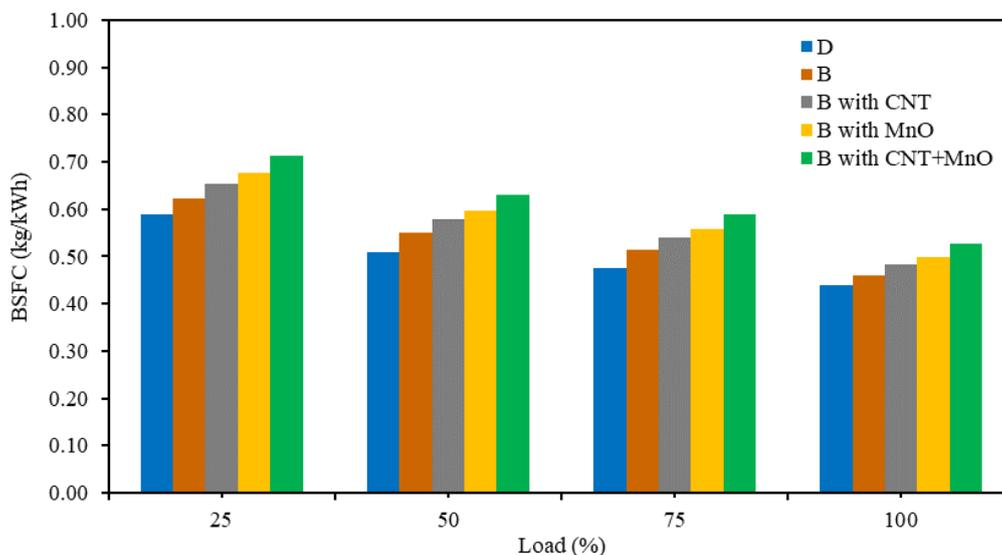
Figure 8. Performance comparison of brake-specific fuel consumption (kg/kWh) and load (%)
