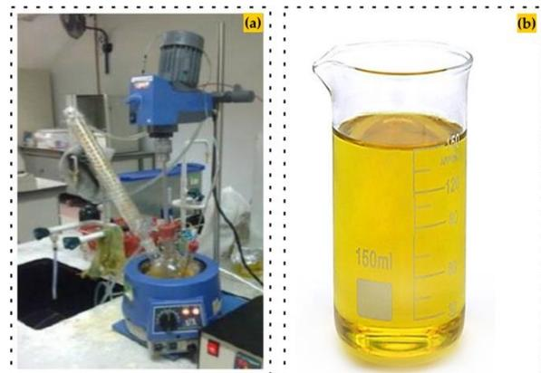
Figure 2. Biofuel preparation (a) Transesterification Process (b) Extracted chicken waste biofuel
