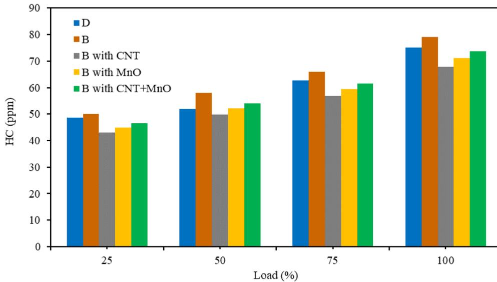
Figure 10. Exhaust emission of hydrocarbons (ppm) variation for the different load (%)
