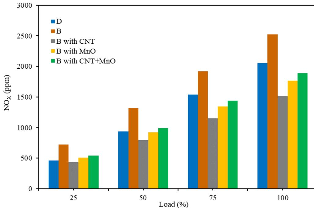
**Figure 12.** Exhaust emission of NO<sub>x</sub> (ppm) variation for the different load (%)
