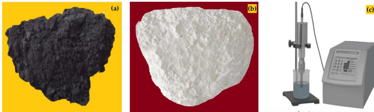
**Figure 3.** Nano fuel preparation: (a) CNT (b) MnO (c) Ultrasonicator equipment
