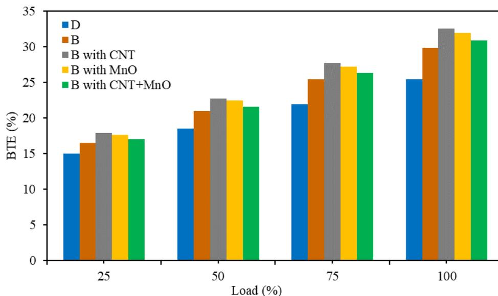
Figure 7. Performance comparison of brake thermal efficiency (%) related to a given load
