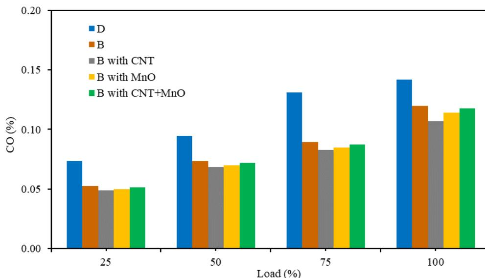
Figure 9. Relationship between exhaust emission, Carbon monoxide (%) and load (%)
