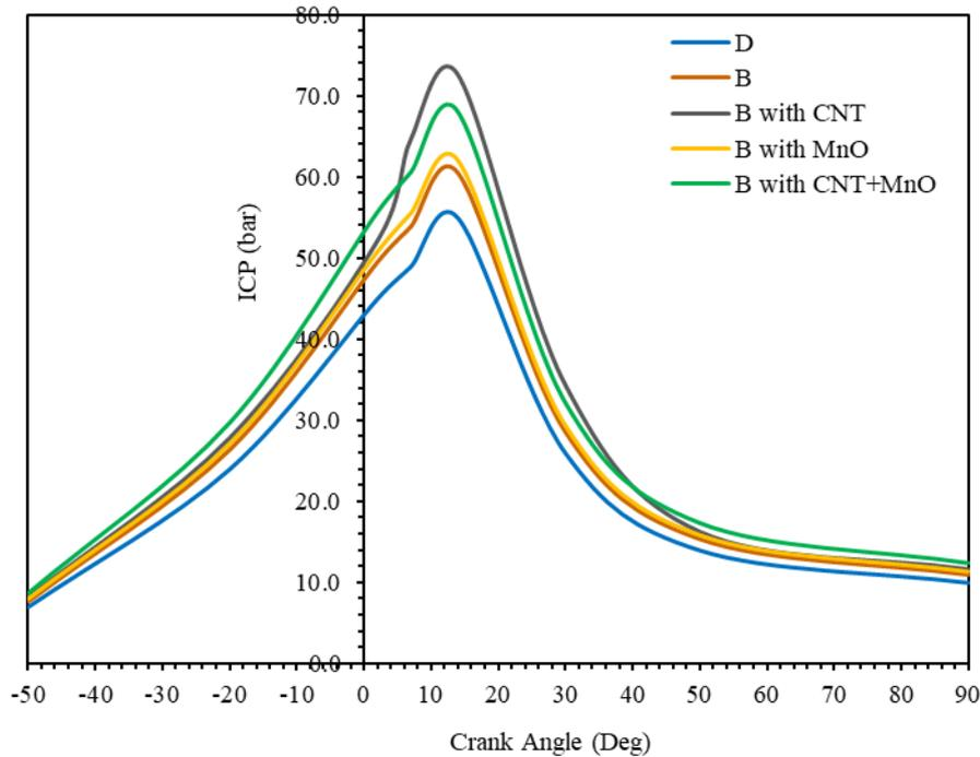
Figure 5. Relationship between in-cylinder pressure, ICP (bar) with crank angle variations (degree)
