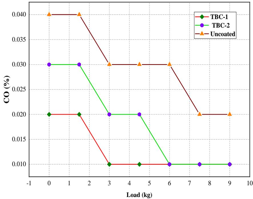
Figure 13. The Difference between coated and uncoated engines' CO emissions
