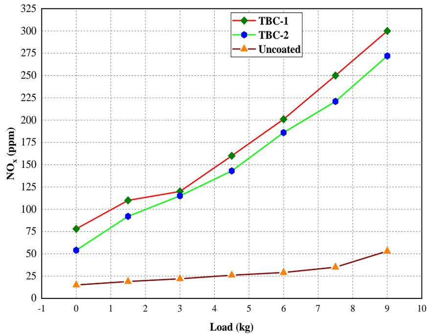
Figure 16. NOx emissions differ between coated and uncoated engines.
