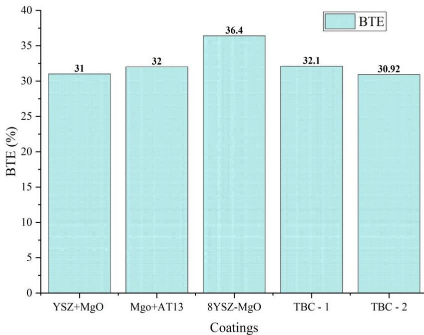
Figure 17. BTE of TBC's engine compared with existing work
