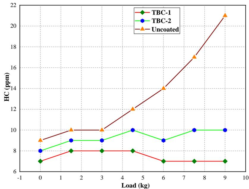
Figure 15. Variation of HC for coated and uncoated engine
