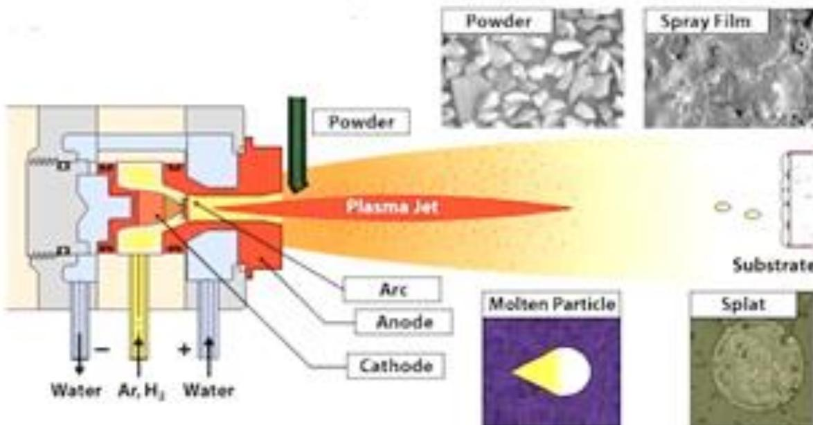
[Figure 1](#). Plasma sprays process
