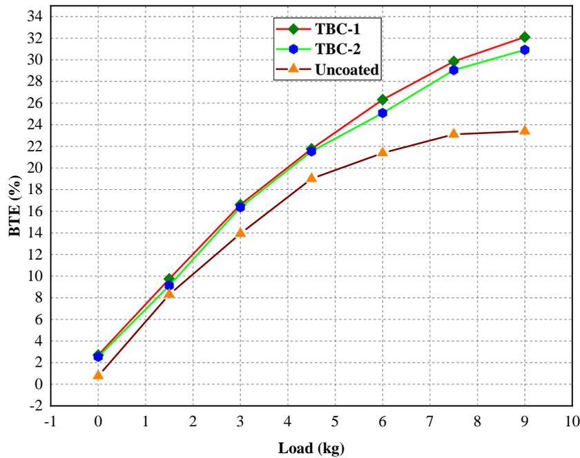
Figure 7. Engine BTE variants with and without coatings
