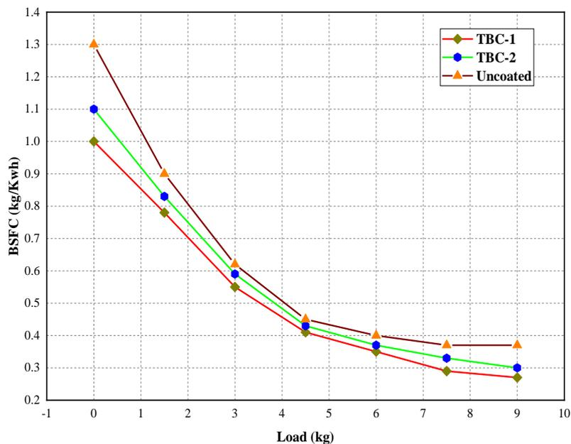
Figure 9. Coated and uncoated engine BSFC variants
