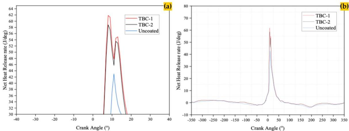
Figure 10. Combustion engine heat dissipation, coated vs. uncoated: (a) engine 1 and (b) engine 2
