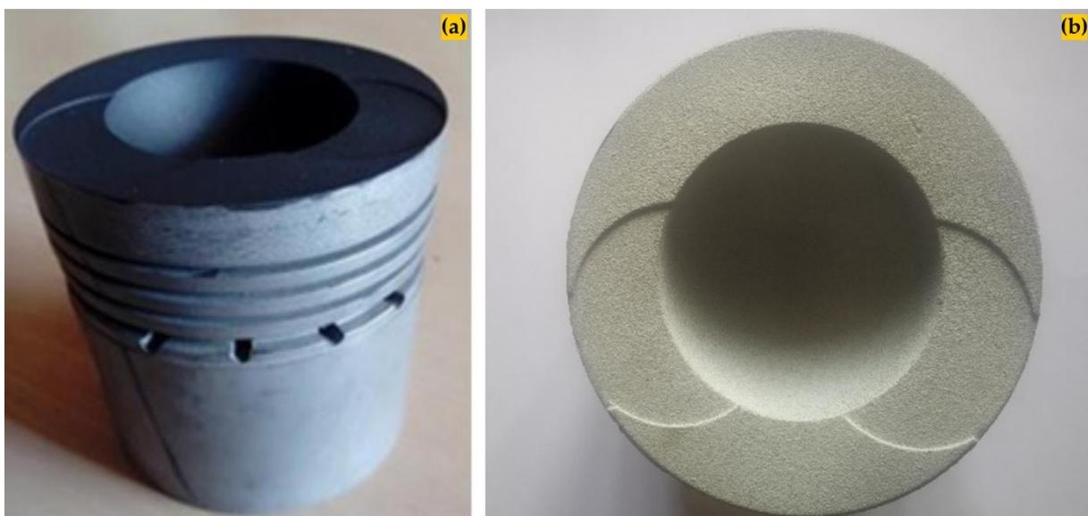
Figure 3. (a) TBC-1 coated piston; (b) TBC-2 coated piston
