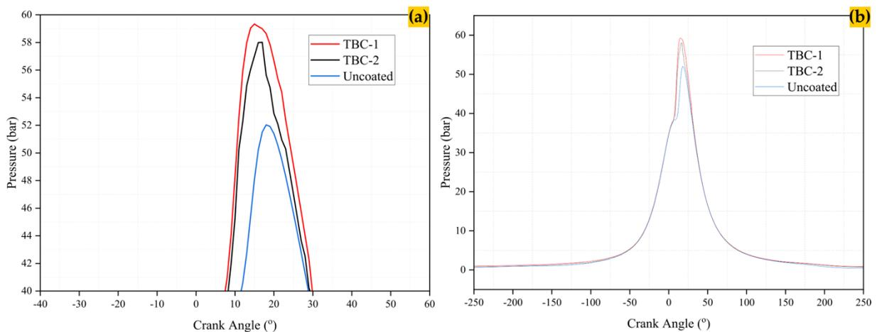
Figure 11. The Effect of Coating on engine pressure: (a) engine 1 and (b) engine 2
