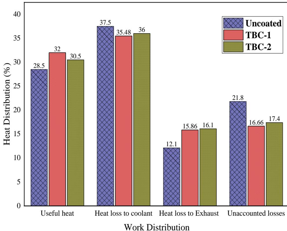
**Figure 12.** Heat balance sheet for coated and uncoated engine
