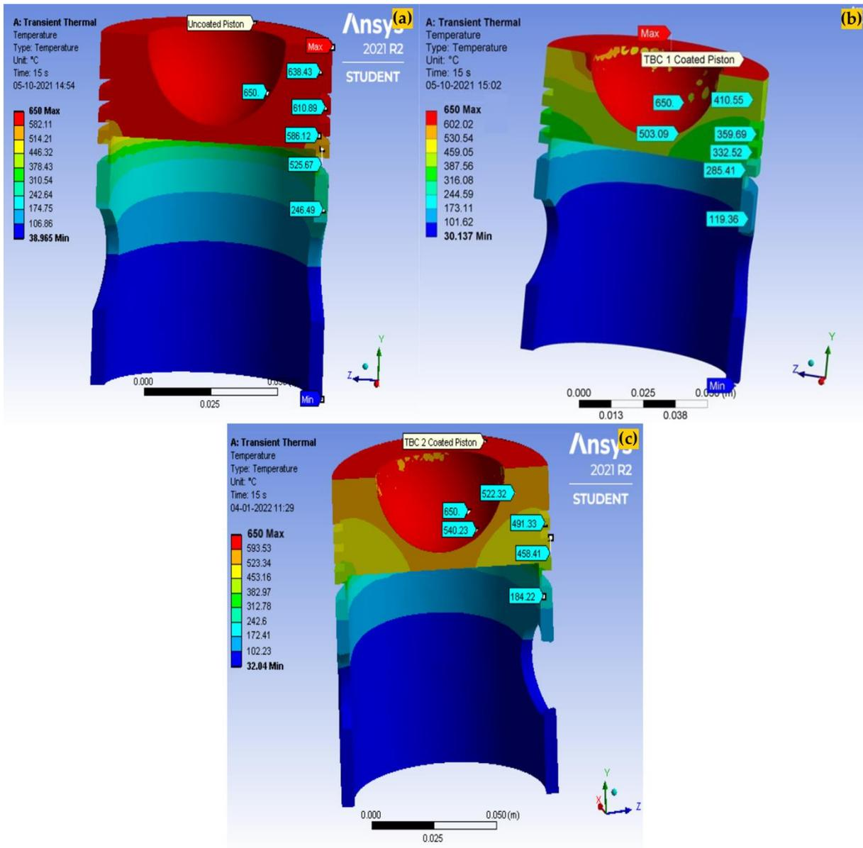
**Figure 5.** (a) Piston temperature distribution when not coated; (b) Temperature profile of the TBC-1 piston; (c) TBC-2 piston temperature dispersion
