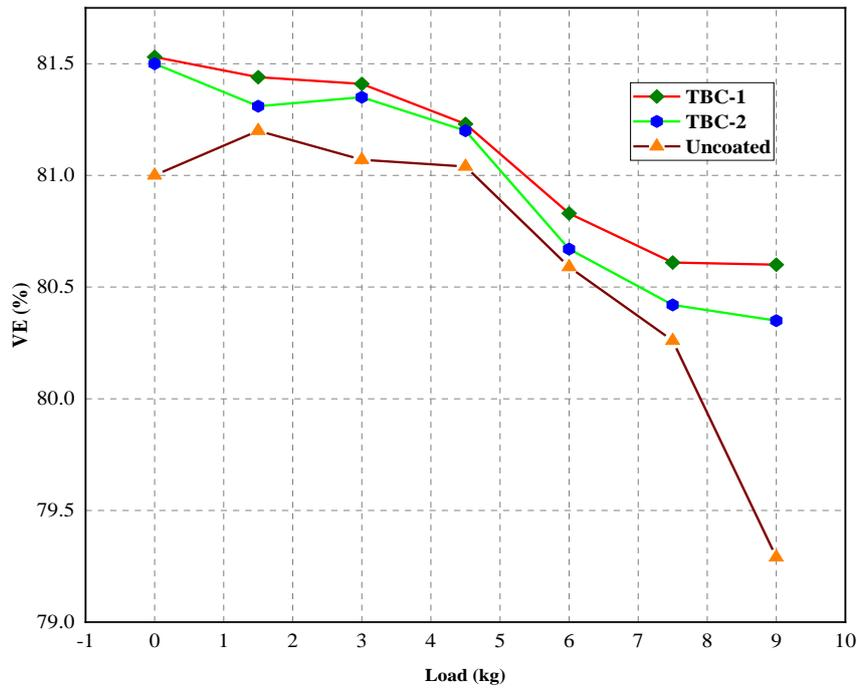
Figure 8. Differences in volumetric efficiency between coated and uncoated engines
