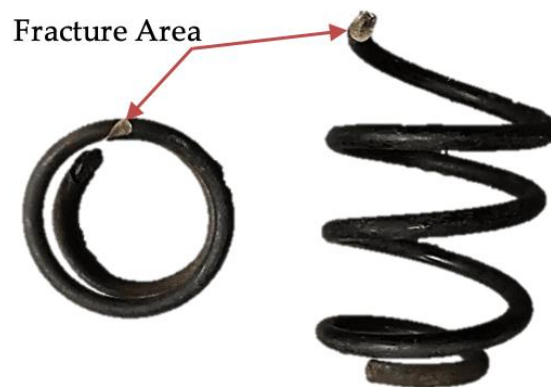
Figure 1. Fracture in coil spring component
