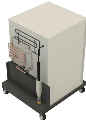
Figure 4. Isometric view of the prototype kerosene-powered vapour absorption refrigerator.
