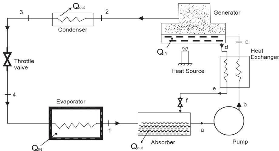
Figure 3. Schematic diagram of the kerosene-powered vapour absorption refrigerator.
