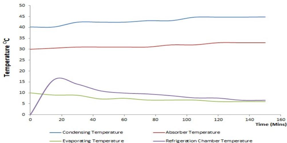
Figure 5. A graph showing the temperature levels at different stages of cooling.
