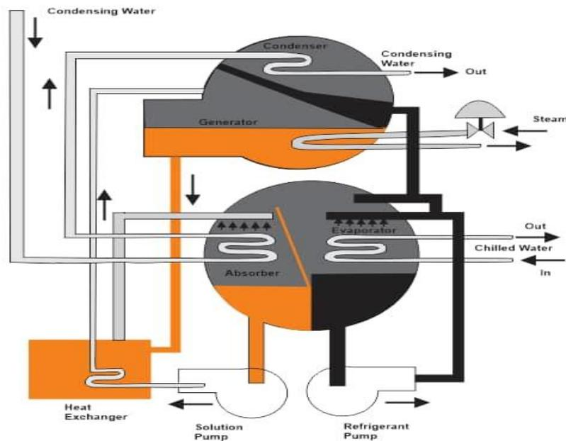
Figure 1. Working of Vapour Absorption Refrigeration System.
