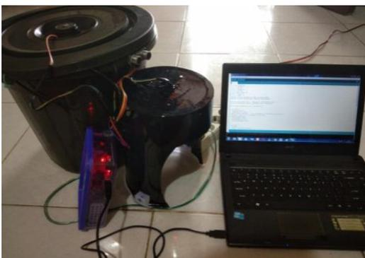
Gambar 5. Rangkaian alat kran cuci tangan otomatis
