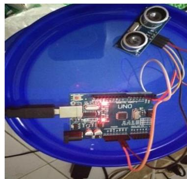
Gambar 6. Pengujian sensor ultrasonik HC-SR04
