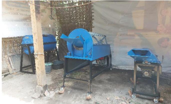
Gambar 4. Mesin pencacah, mesin rotary kiln / compost barrel
