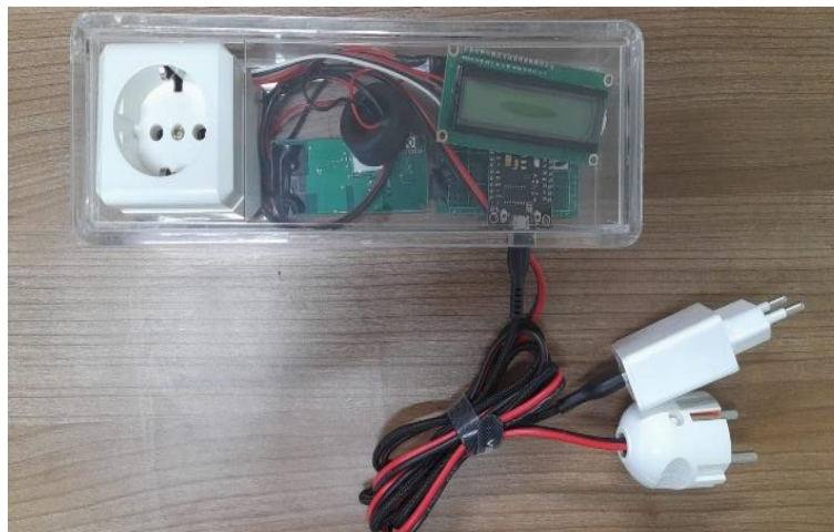
Figure 1. The IoT-based prototype of electricity monitoring system
