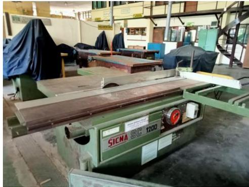
[Gambar 2](#). Mesin gergaji (*circular saw machine*)
