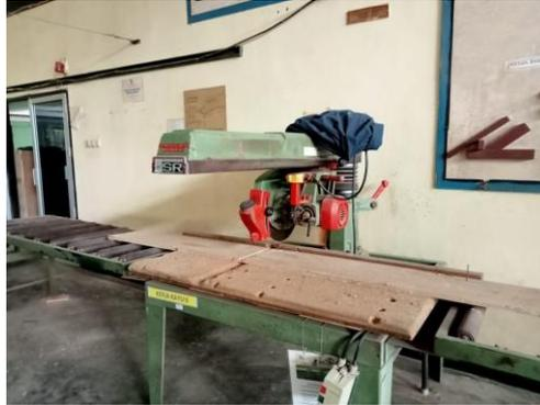
[Gambar 1](#). Mesin gergaji potong (*radial arm saw machine*)
