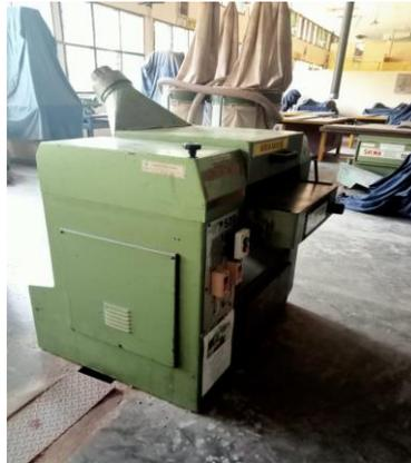
Gambar 3. Mesin ketam penebal (*thicknessing machine*)
