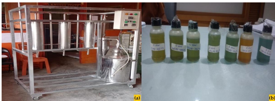
Figure 2. The pyrolysis process for plastic waste: (a) Plastic waste pyrolysis machine; (b) Variation in the mixture of PPO: Gasoline
