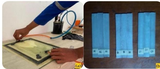
using a vacuum pump with a pressure of 68 cmHg. The composite was dried for 3 days at room temperature ± 25°C and given a Code to prepare for testing in the laboratory, as shown in **Table 2**. To ensure the accuracy of the data in this research, each sample was molded three times.
