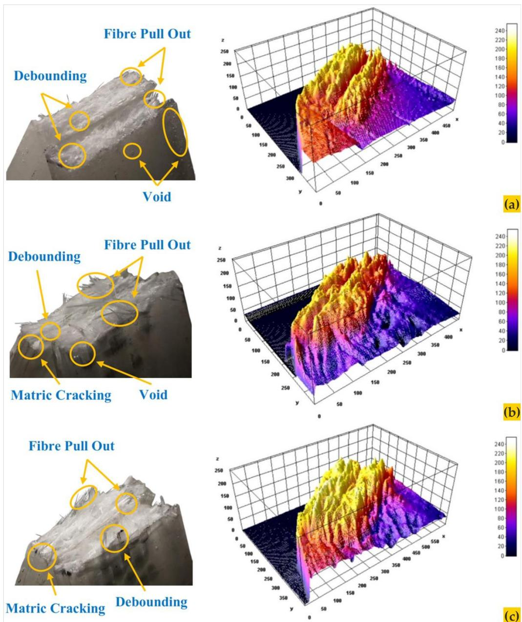
**Figure 8.** Fracture macro and imageJ analysis: (a) CSM; (b) WR; (c) WC
