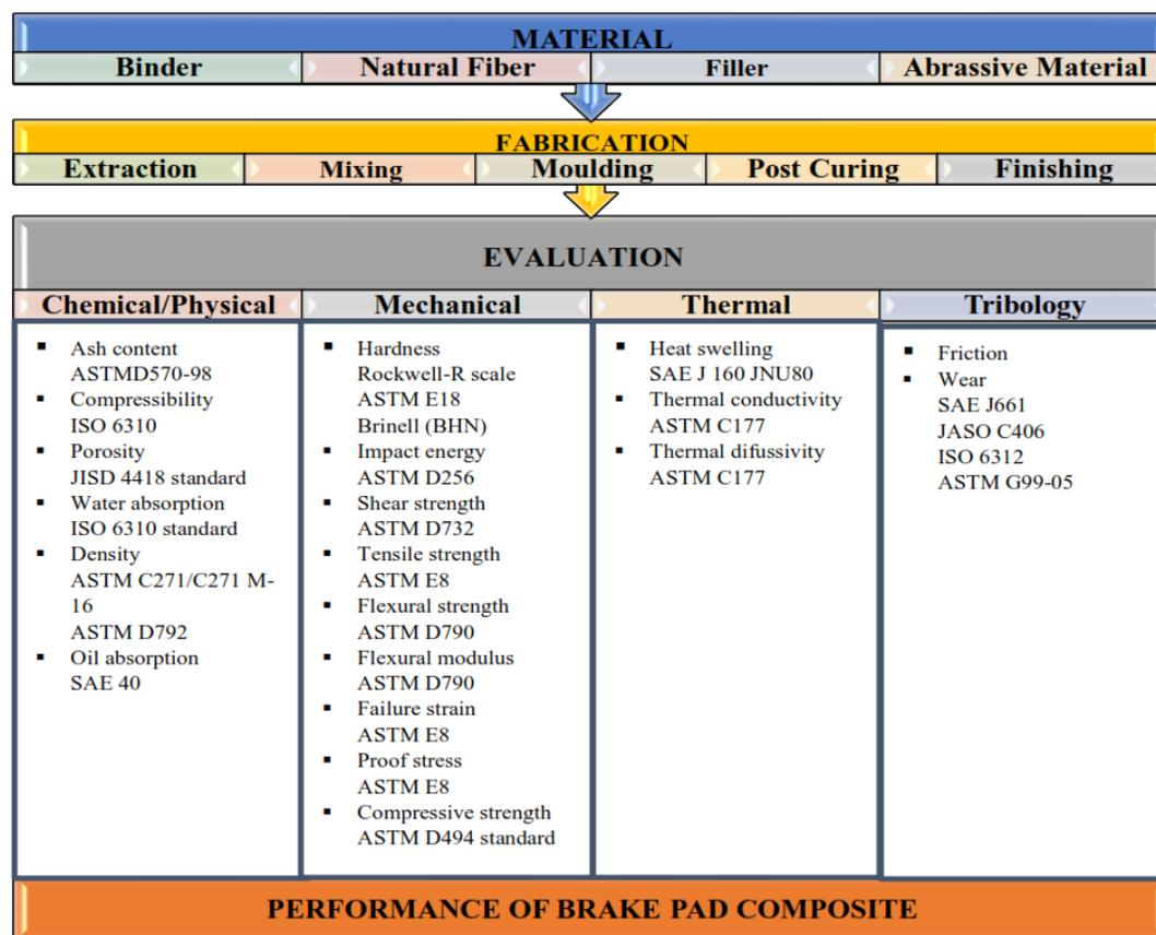
Figure 6. Manufacturing flow of brake pad composite
