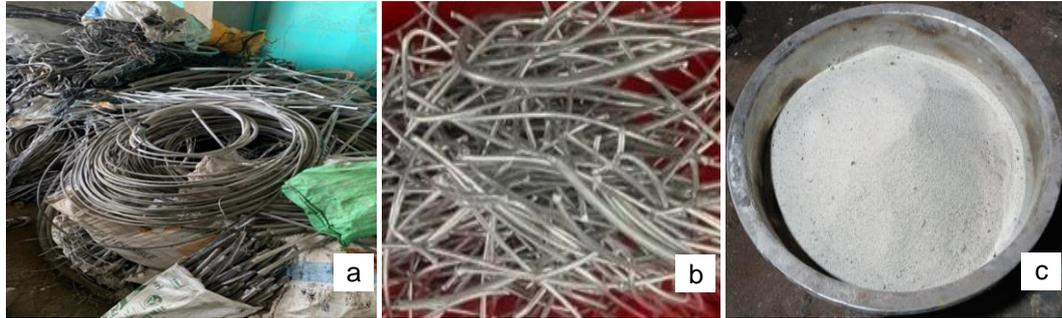
**Figure 1.** The materials used in this study: (a) Electrical cable before cutting, (b) Electrical cable cut to 20 cm; and (c) Silica sand
