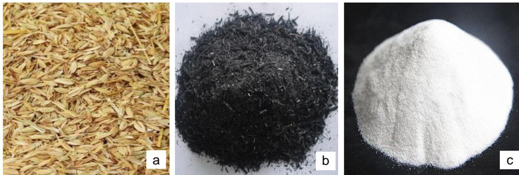
**Figure 2.** Rice husk ash (RHA); (a) Rice husks, (b) Rice husks after burning at 400°C, (c) Rice husk ash after heating at 900°C for 2 hours
