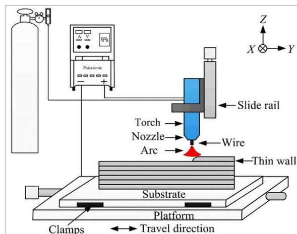
Figure 1. Schematic of WAAM process [5]
