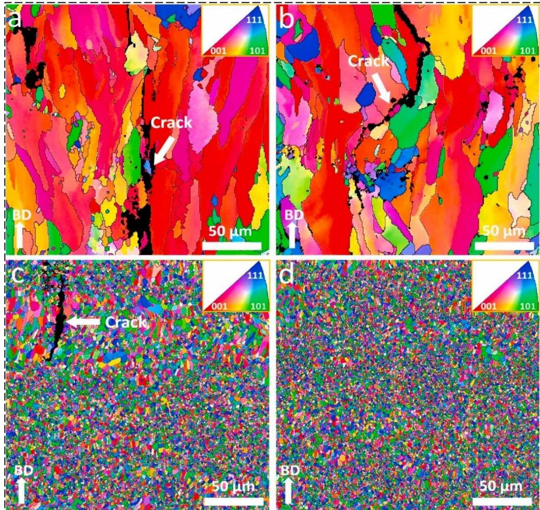
**Figure 3.** Longitudinal EBSD inverse pole figure (IPF) maps are shown for the following samples produced with an energy density of  $83 \text{ J/mm}^3$ : (a) 7075; (b) 7075-AS; (c) TI-7075; and (d) TI-7075-AS. The maps illustrate crystal orientations along the build direction, with the IPF color code indicating the grain orientations [28]
