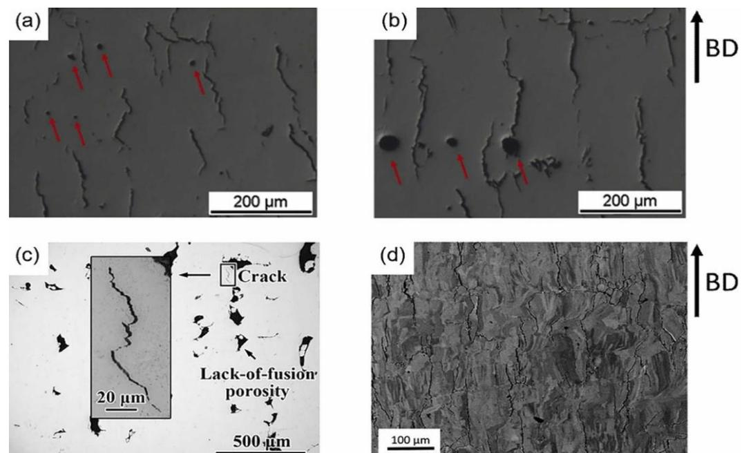
**Figure 7.** Two kinds of defects in AM of aluminum alloys: (a-b) Spherical pores with different sizes [66]; (c) irregular holes due to lack of fusion and solidification cracks [67] and; (d) solidification cracks [66]
