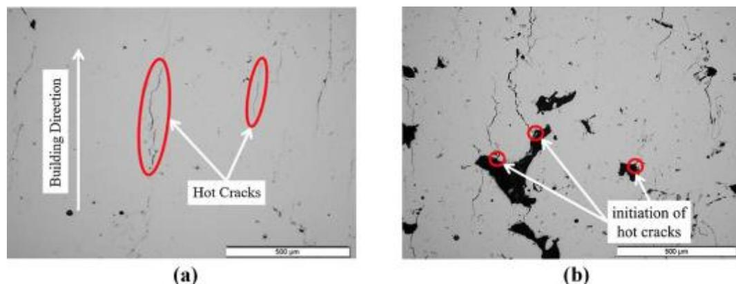
**Figure 6.** Cracking in AMed parts: (a) SEM microscopy of hot cracking in SLMed AA7075 with 500 W laser power and 1200 mm/s scanning speed [24]; (b) Porosity formation and hot crack initiations due to porosity of SLMed AA7075 [24]
