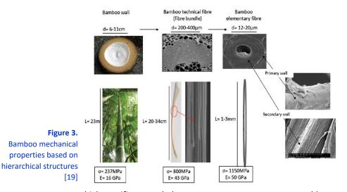
Bamboo as a plant or its fibers represents a natural composite due to its structures comprising matrix and reinforcement as shown in Figure 3. Bamboo fibers, extracted from its culm, are comprise of technical (100~200 microns) and individual (< 30 microns) fiber forms [19], [20]. Bamboo fibers have the potential to utilize as reinforcement for environ-mentally friendly compo-sites due to their
