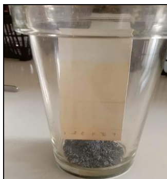
Figure 4. Silica gel plat evaporation using Iodin cristal vapor for fatty acid detection
