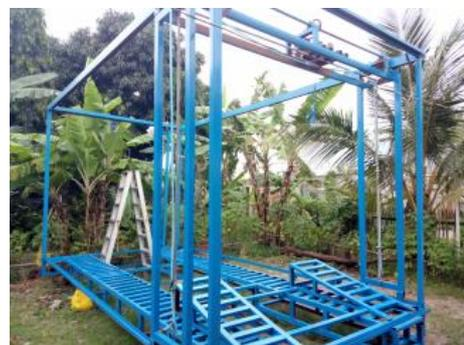
**Gambar 1. Rangka Mesin Cuci Mobil**
