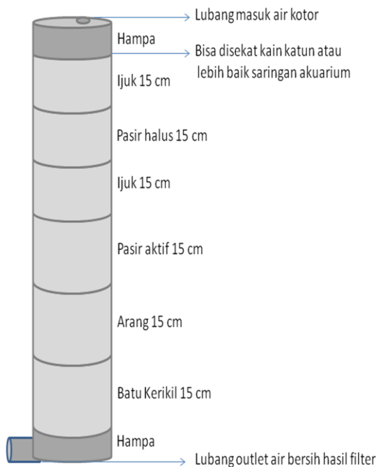
Gambar 6. Skema Filter Air Sederhana
